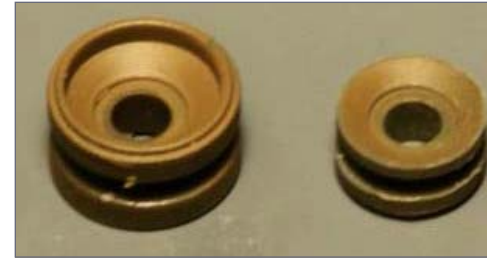
56. A stock roller on the left compares to a roller on the right that has been reduced in size.
