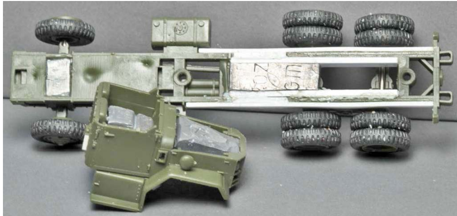
12. Weights added between the truck frame and in the cab body.
