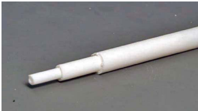
18. Forming the drive hub from tube styrene.
