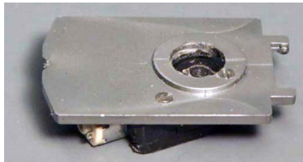
23. Cab turntable drive viewed from the bottom.
