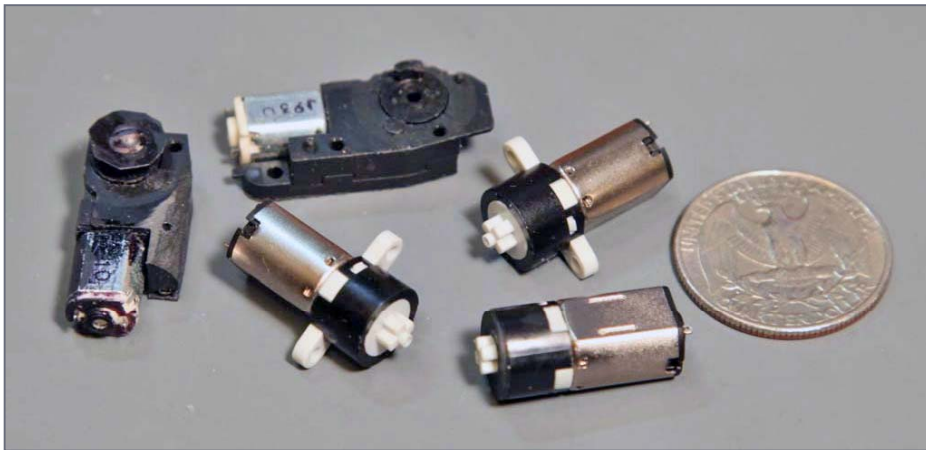
38. The planetary-gear drive motors for crane 19. The quarter gives you a good idea of how small these motors are.
