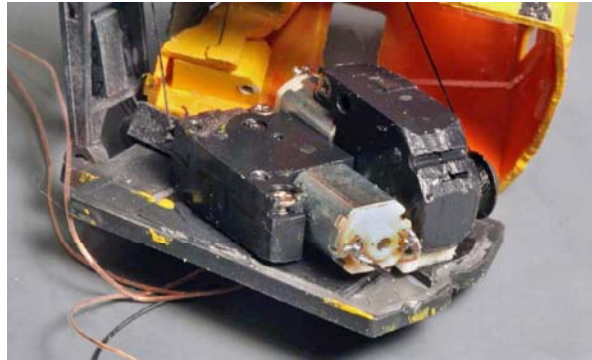
28. Cab turntable drive motor (left) and hoist motor (right).
